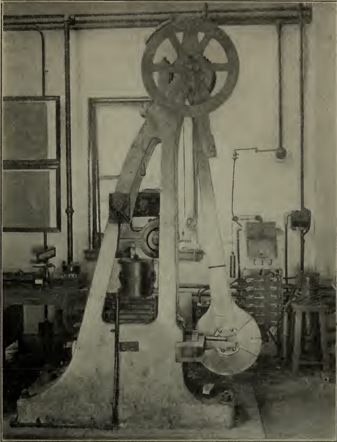
FIG. 23.—Charpy Impact Testing Machine Used by Langenberg.
